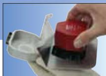
Circulating nurse presses the non sterile battery into the battery housing.
