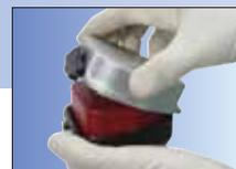
Sterile scrub technician closes battery housing lid and secures locking knob.
